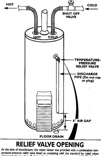
perature-pressure relief valve listed as complying with the standard for relief valve and automatic gas shut-off devices for hot water supply systems, ANSI Z21.22. For safe operation of the water heater, the relief valve must not be removed from its designated point of installation or plugged.
